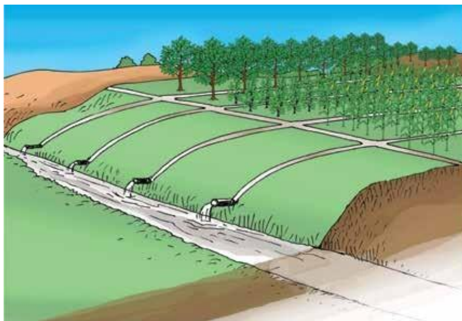
Figure 6.13 Drainage Channel (Source: Godinho et al. , 2023)
